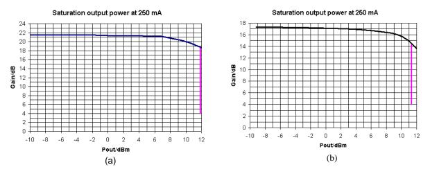
Fig. 2 Typical saturation output power as shown by the magenta line at 250 mA for:
