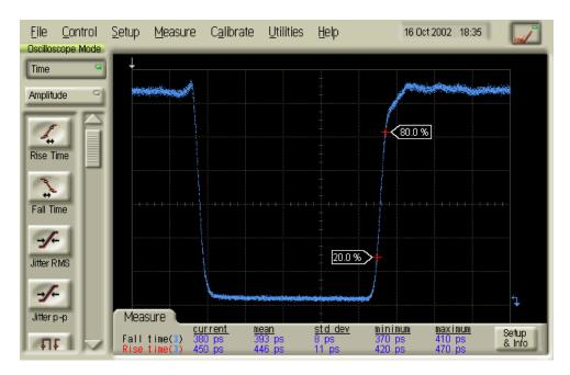
Fig. 5 Typical switching time for IPSAD1302 and IPSAD1502 SOA Devices
