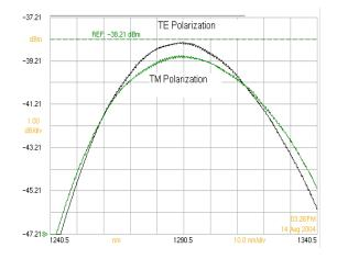
Fig. 4 ASE spectrum power for TE and TM polarization at 250mA measured on an InPhenix IPSAD1301 SOA.
