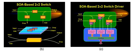
Fig. 10 (a) SOA-based ROADM, (b) Three SOA gates are required per wavelength channel, (c) Driver diagram for SOA-based gate switch in ROADM.
